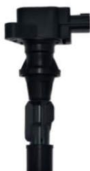
Ignition Coil for Mazda 3 6 Sport MX-5 CX-7 L4 2.0L 2.3L 2.5L 6M8G-12A366
