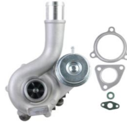
Right Side Turbo Charger for Ford Flex Taurus SHO Explorer Sport Lincoln MK...
