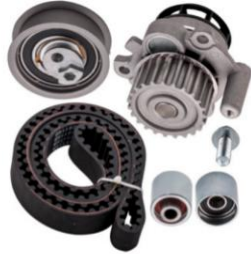
Timing Belt Kit W/Water Pump Fit for Audi A3 A4 TT 2009-2014 For VW...
