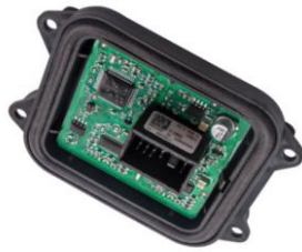
Performance Headlight Controller Diver Module For BMW E90 E91 E92 E93 X...
