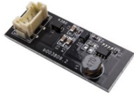
Rear LED Tail Light Driver b003809.2 Board Chip Replacement For BMW X3...
