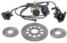
Rear Brake Master Cylinder Kit Universal for Go Kart 150cc for KD150BRKIT
