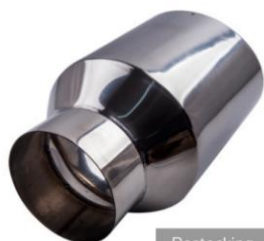
5 inch Inlet 8" Outlet 15 inch Long Rolled End Angle Cut Exhaust Tip Tail...
